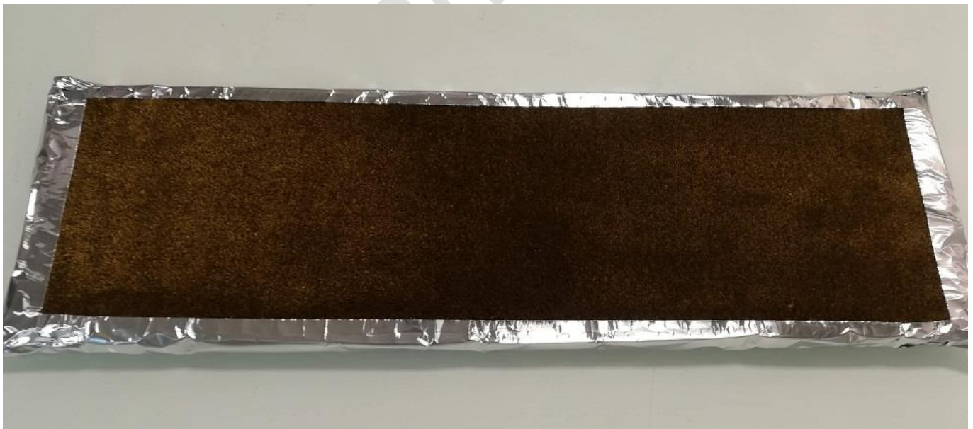
Figure 1 : Test specimen of the 100% 6.6 NYLON (SBR Latex) carpet
